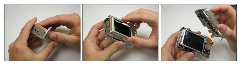
• Gently lift the rear of the case to remove it from the camera.
