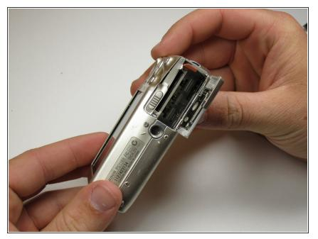
• Remove the battery and SD card from the camera.
