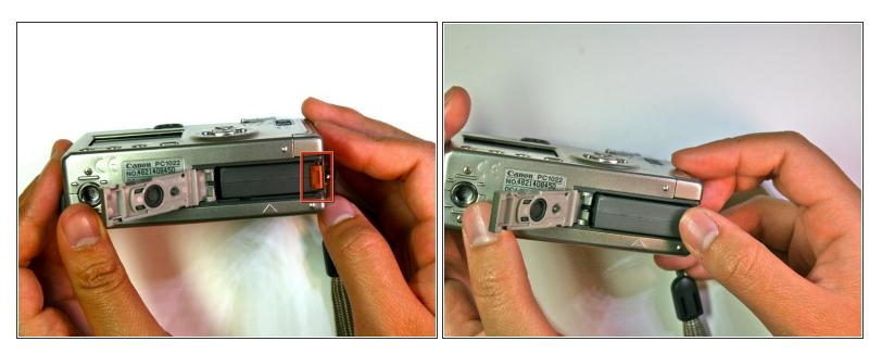
• Push and slide the orange retaining clip to the right to remove the battery.
