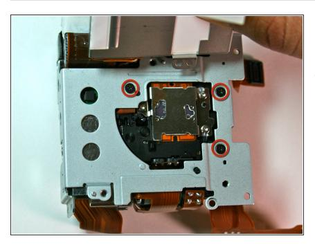
Remove the three (3.1mm) black screws that were behind the screen and battery box.
