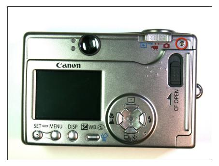
• Remove the 3.8mm screw from the back face of the camera.
