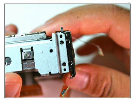
Carefully pry the left side of the housing plate from the bottom of the tripod mounting plate, releasing it from the two alignment pegs next to the screws
