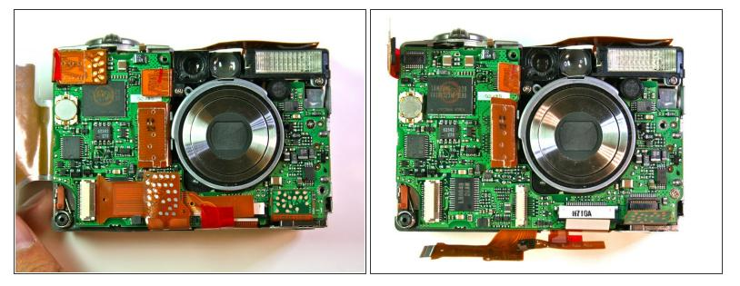
• Remove the wire connections that connect along the bottom of the motherboard.
