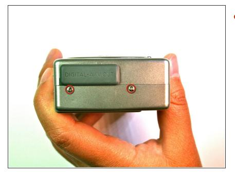
Remove the two 2.3mm screws from the right face of the camera.
