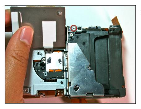
Remove the card-reader shield by removing the screw at the top of the shield.
