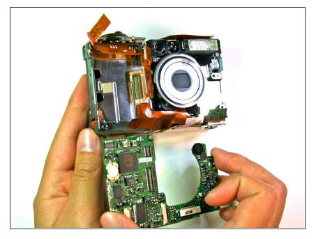
• Remove the motherboard from the main frame of the camera body.
