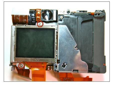
Remove the 2.1mm screws from the bottom and top of the screen connecting it to the housing plate
