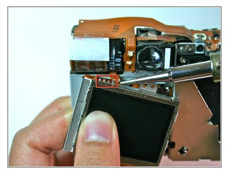
• Unsolder the four points at the top of the screen with a soldering iron
