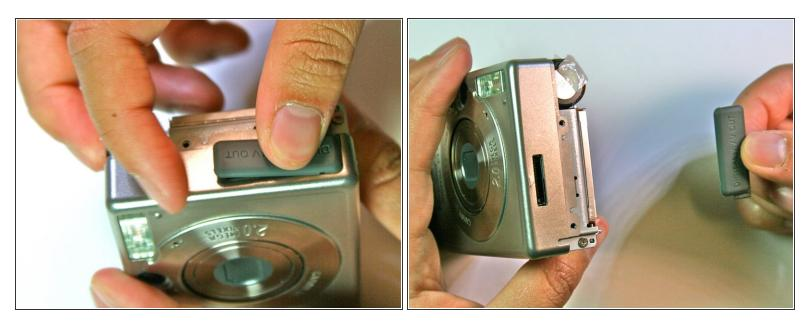
• Slide the rubber digital a/v cap out of place on the front plate.
