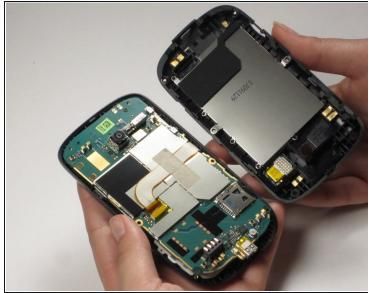
Carefully pull off the back casing.
