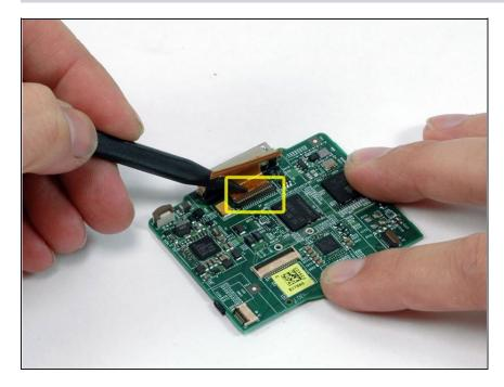
• Use a spudger to flip up the plastic tab holding the orange hard drive ribbon in place. The tab will rotate up 90 degrees, releasing the ribbon cable.
