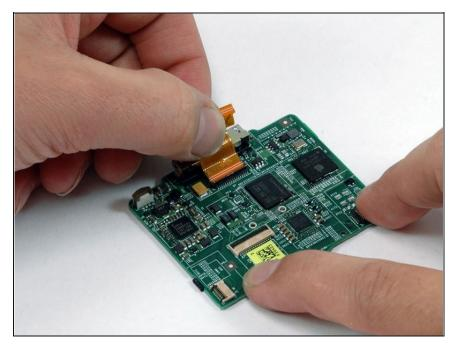
Slide the orange hard drive ribbon cable directly out of its connector. The cable may be attached to the logic board with some adhesive. If the cable doesn't immediately come free, carefully pull up on the cable to loosen the adhesive.
