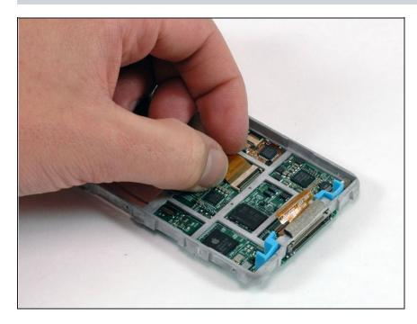
• Slide the orange display ribbon cable directly out of its connector.
