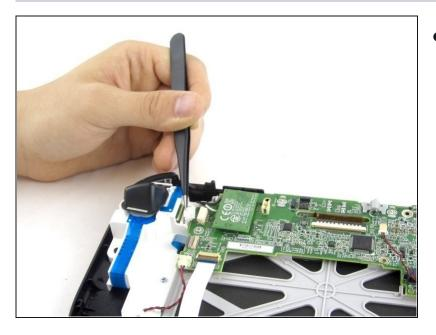
• Disconnect the analog connector with tweezers.
