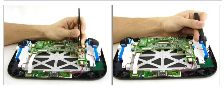
• Remove the right speaker cable that's connected to the motherboard with the tweezers.
