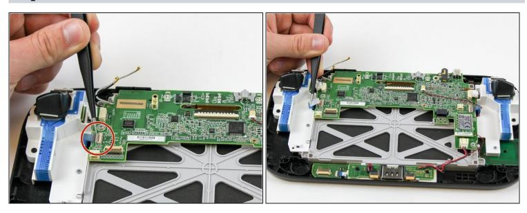
• Remove the blue connector using tweezers.
