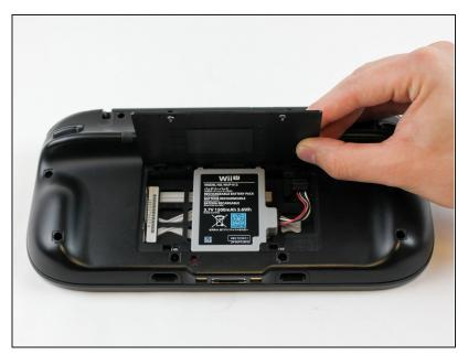
• Lift and remove the battery plate.
