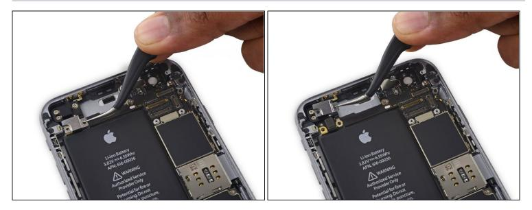
• Remove the upper component cable connector bracket.
