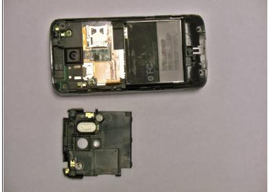
Lift the plastic cover near the memory card slot.
