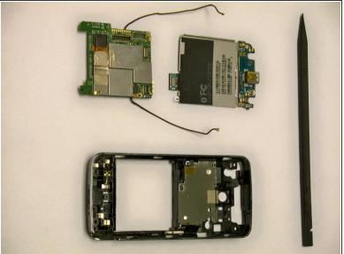
Gently lift the motherboard up using a nylon spudger.
