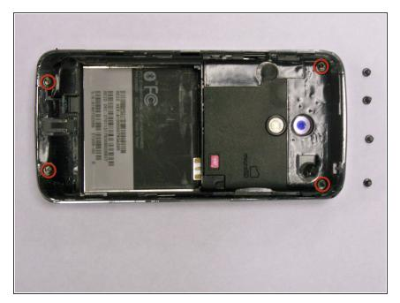
Remove the 4 screws using the T6 screw driver.
