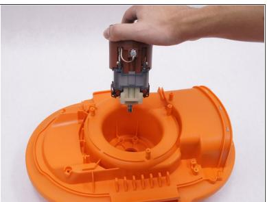
• The motor is ready for replacement. Pull the motor to separate.
