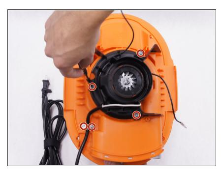
Remove the five 15mm screws from the plastic motor cover and power cord clamp using a PH2 screwdriver.
