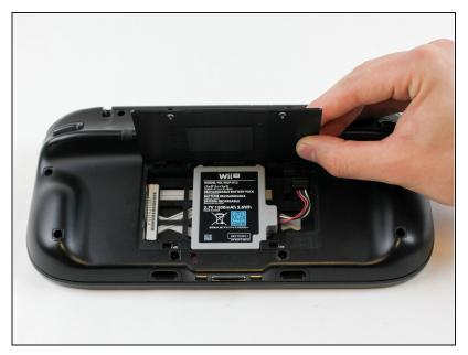
• Lift and remove the battery plate.
