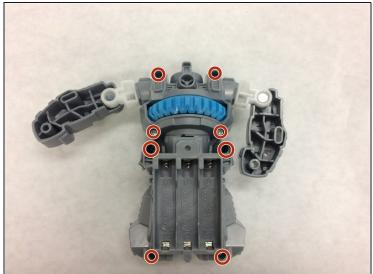
Using a Phillip #0 screwdriver to remove the eight 8 mm screws.
