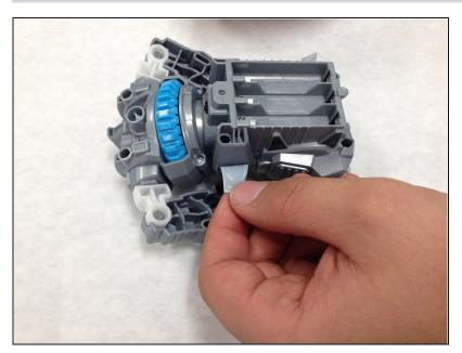
Peel back the four decal stickers that hold the front and back of the bot together.
