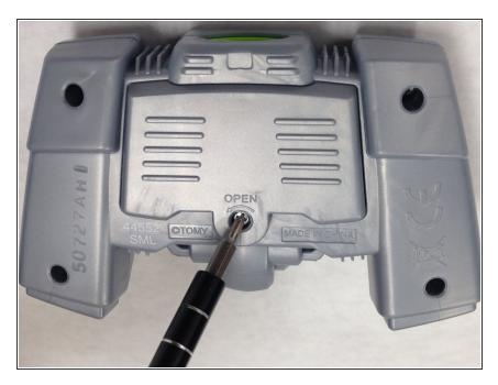
Remove the screw on the battery lid.
