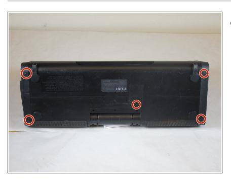
Remove the five screws on the underside of the device using a PH0 screwdriver.
