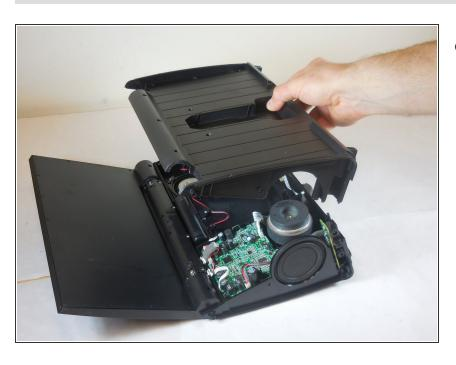
At this point, the back panel of the device should lift off easily. Lift it off and set aside.
