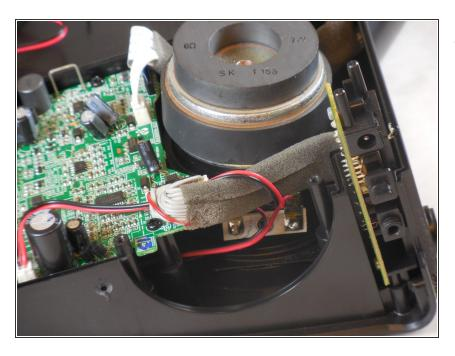
Inspect wires and locate any speaker loose connections.
