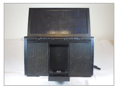
Extend the solar panel into the upright position to access the screws on the backside of the device.
