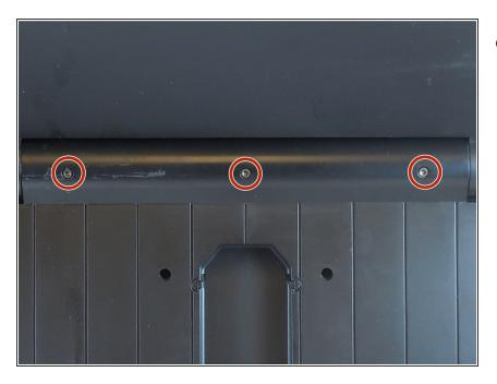
Remove the three screws at the top of the back panel using H2.5 hexagonal screwdriver.
