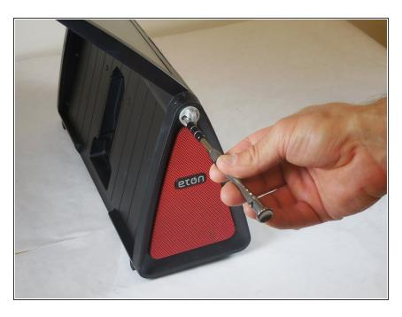
Remove two screws from each side using a H2.5 hexagonal screwdriver.
