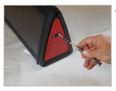
Remove the two screws that were covered by the "Eton" logo using a PH0 screwdriver.
