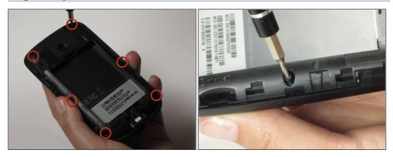
• To remove the back casing inside the phone, remove the six screws around the perimeter.
