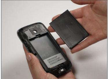
• Insert your finger or a pry tool into the slot above the battery. Remove it and set aside.
