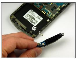
↑ There is a wire under the antenna connecting it to the Motherboard. Do not pull off the antenna just yet.
