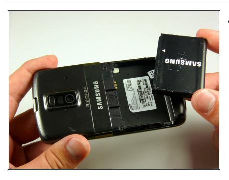
Grasp the bottom left and right corners of the battery and lift it from its housing.
