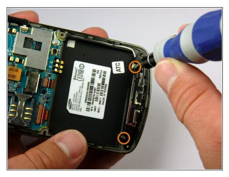
Remove the two silver 4.30 mm screws on either side of the antenna using a Phillip's #00 Screwdriver.
