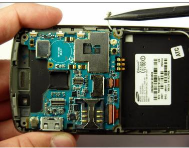
Use a spudger to disconnect the white antenna wire on the bottom right corner of the Motherboard.
