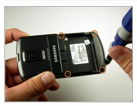
Remove the four black 7.30 mm screws surrounding the battery housing using a Phillips #00 Screwdriver.
