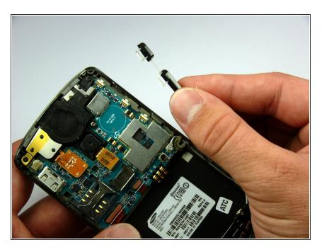
Remove the power and volume buttons on the right side of the Motherboard.
