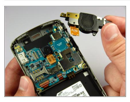
Lift the speaker out of its compartment.
