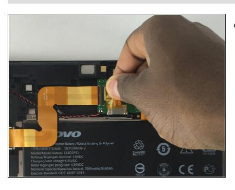
Remove the second piece of tape from the other ribbon cable connected to the battery.
