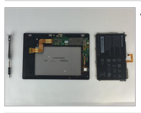
Once the battery ribbon cable is detached, carefully remove the battery.
