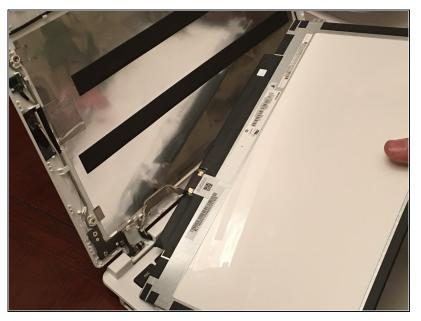
Pull the ribbon cable out with tweezers and remove the screen.
