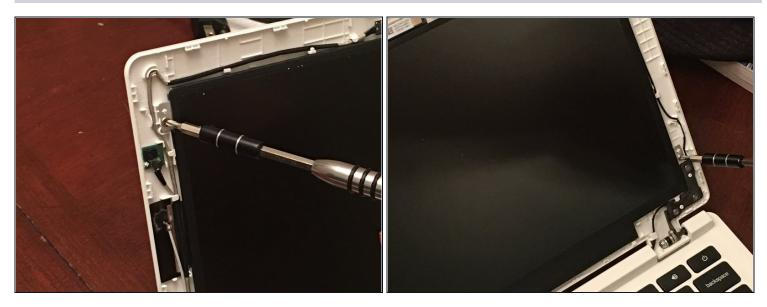
Remove the four screws within the silver brackets that are holding the screen to the back of the laptop.
