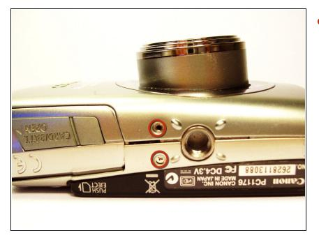
Remove the two, small screws on the bottom of the camera using a Phillip's #00 screwdriver.
