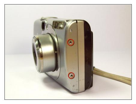
• Use a Phillips #00 screwdriver to remove the two, small screws on the right side of the camera.
