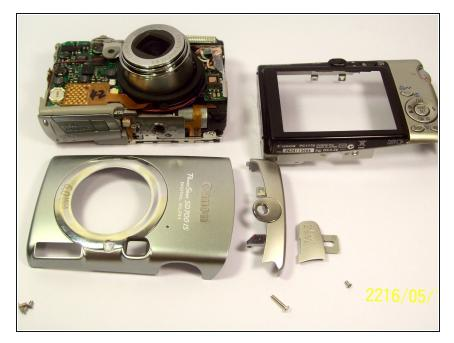
• Remove the front, back, and side casings from the camera and set to the side.
