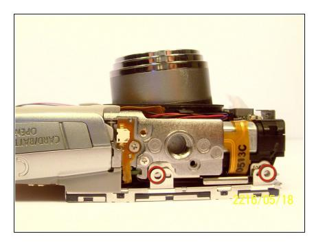
• Remove the two screws that connect the LCD and backlight to the main body of the camera.
