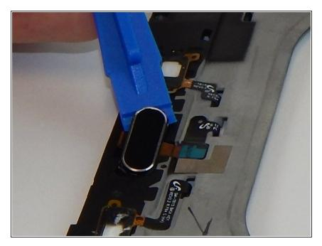
Flip the device open and gently pry the home button out using the plastic opening device.
