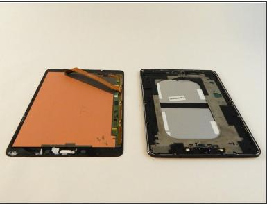
With the plastic opening tool gently lift to disconnect the gold ribbon cable that attaches the screen to the base tablet.
