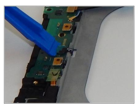
Using the plastic opening device detach the rear connector of the home button from the device.
