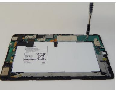
Remove the four black 3 mm Phillips #1 screws that hold the battery in place.
