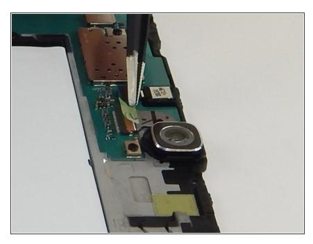
Remove strip of green tape covering the camera connector with the tweezers.
