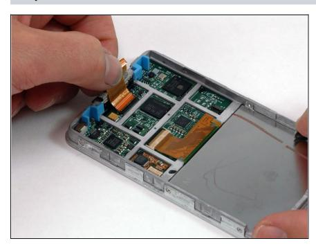
Slide the orange hard drive ribbon cable directly out of its connector. The cable may be attached to the logic board with some adhesive. If the cable doesn't immediately come free, carefully pull up on the cable to loosen the adhesive.
