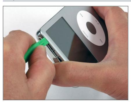
Near the other top corner, insert a plastic opening tool into the seam between the front and back of the iPod
