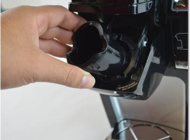
Once all of the tabs have been pressed, the K-Cup should just pop out. After, you just pull the remainder of the K-Cup. You have successfully removed the K-Cup.
