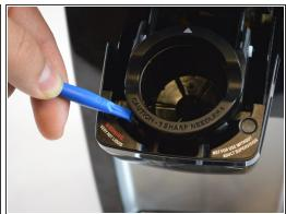
Press on tab while pulling up on K-cup until you hear a click. Repeat for the remaining tabs. We found using the smallest of the "plastic opening tools" worked wonders.
