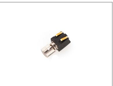
The vibrator is only fastened by the plastic bracket.
