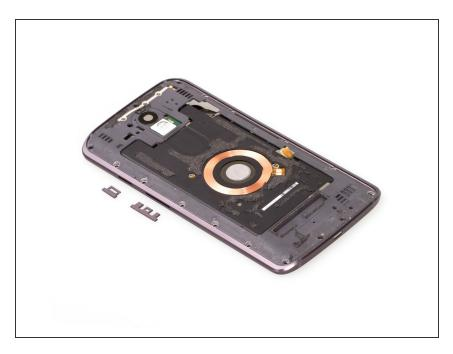
After middle frame's separating from the rest of parts, side buttons are loose and easy to remove.
