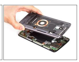
Take away rubber bracket securing MIC flex and release microphone flex cable connector.
