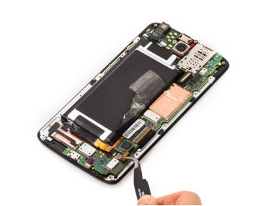
The LCD assembly has two connectors, here is touchscreen connector.
