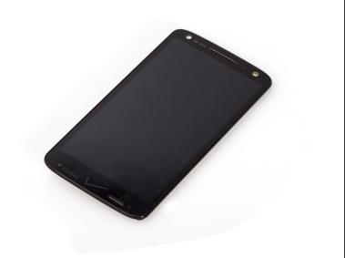
Here is LCD screen with LCD supporting frame. They are attached tightly, so we haven't separate them.
