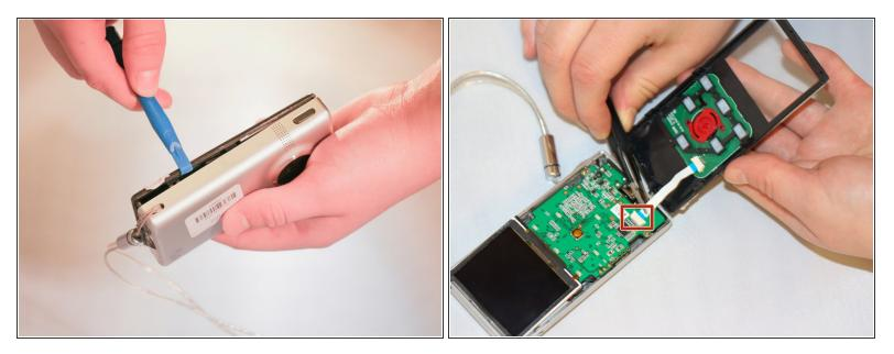
• With the plastic opening tool, gently pry the front casing away from the device by carefully running the tool around each edge and lifting.
