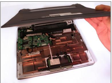
Use a plastic prying tool to take off the bottom case. Make sure that all of the clips are unclipped before trying to remove the case.
