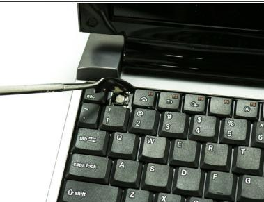
To take off the Keyboard there are three tabs at the top of the Keyboard in the locations shown in the picture that you must press and unclip. They are located behind each of the keys that are removed.
