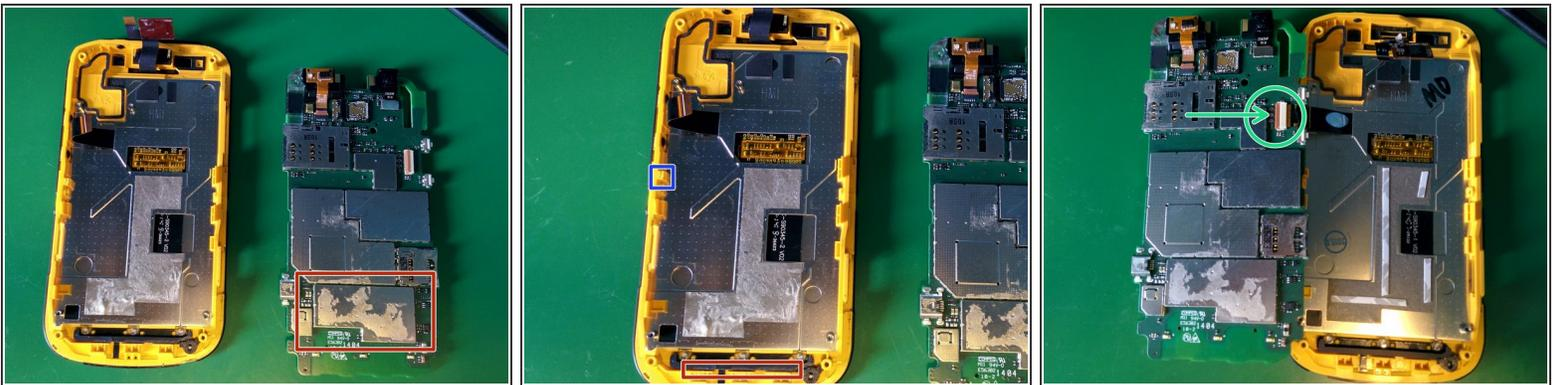
**⚠** Be careful of LCD connector on the underside of the board through all of these steps (see green).
