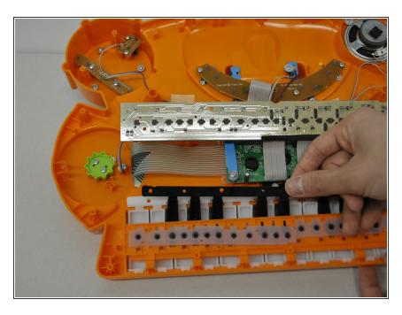
Pull out the black piano keys and replace with the new piano key part.
