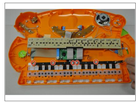
Unscrew 6 PH2 screws (11 mm) on the black bar holding the keys on the device.
