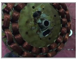
Use three sockets to level the rotor core, while giving the bearing a final push.
