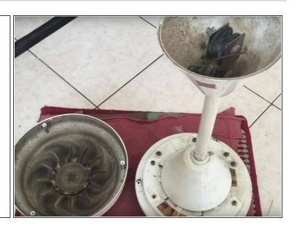
First, unscrew the mounting screw for the plastic cover located along the brim furthest from the centre.
