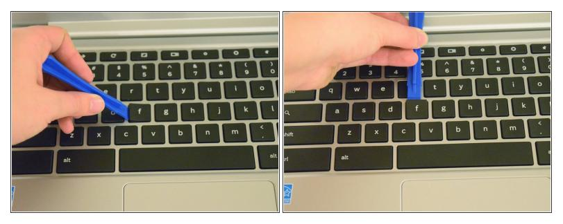
• Using a plastic opening tool, place it beneath the key in question and pry it off.
