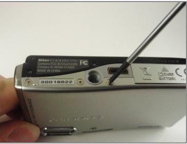
• Remove all five screws from the bottom of the camera using a Phillips #00 screwdriver.
