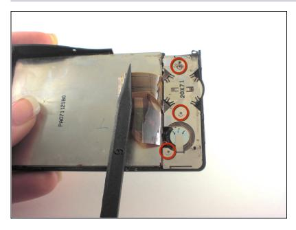
On back of LCD screen, locate the three screws underneath the ribbon and remove them.
