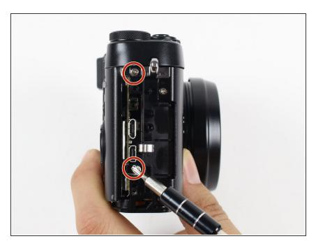
Remove the two 6.0 mm screws beneath the port cover assembly.
