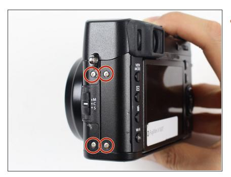
Remove the four 5.0 mm screws on the side of the camera that is opposite to the battery.
