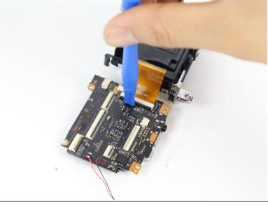
• Use the plastic opening tool to remove the orange ribbon on the motherboard by wedging the tool under the ribbons black tab, and carefully prying upwards.
