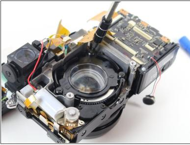
Remove the three 3.5 mm screws on the spring-loaded cover.
