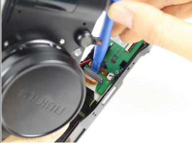
• Use a plastic opening tool to detach the two ribbon cables from the top frame.
