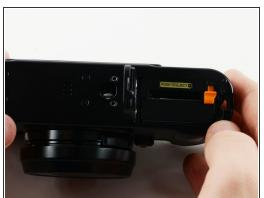
Slide the small black tab on the bottom of the camera to the left to unlock the battery cover.
