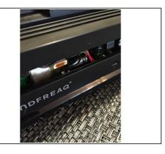
Now you can carefully pull the back frame of the speaker away from the main body. Don't fully separate them before taking care of the electrical connectors on the left, right, and top sides of the speaker. After they're all disconnected, fully separate the back plate from the frame.
