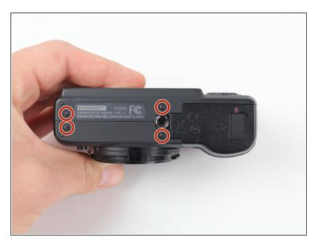
Remove the four 3.3 mm screws on the bottom of the camera using a Phillips #00 screwdriver.
