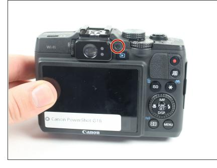
Remove the 3.3 mm screw on the right side of the viewfinder using a Phillips #00 screwdriver.
