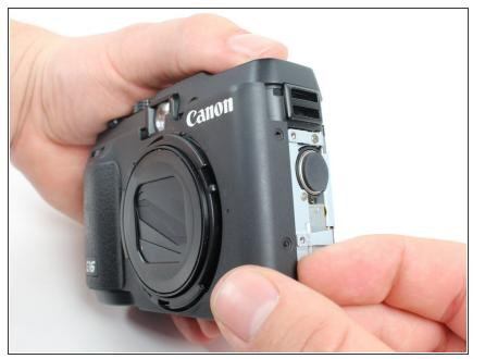
• Using your fingers, carefully pry the front cover off starting at the bottom right.
