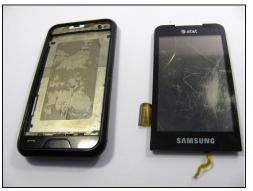
• Use a small tool to pry the digitizer and screen (together) from the frame of the phone. This may take some time and careful work because it is glued down to the frame.
