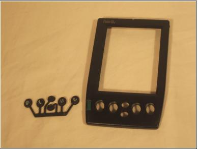
Using a prying tool, carefully pop button pad out of the cover.
