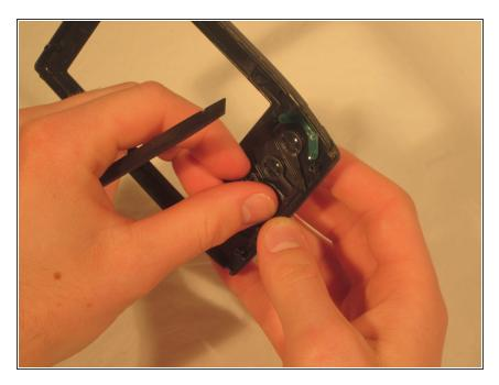
Insert the new button pad where the old one used to be.
