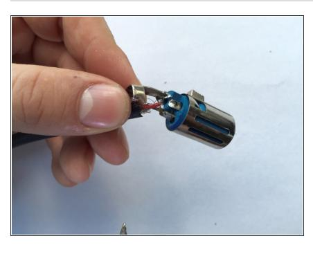
Assess which connections have fallen loose. In this instance, the white cable is disconnected.
