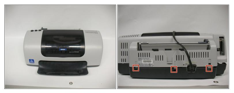
• To remove the top cover of the printer, you have to first release it from several tabs.
