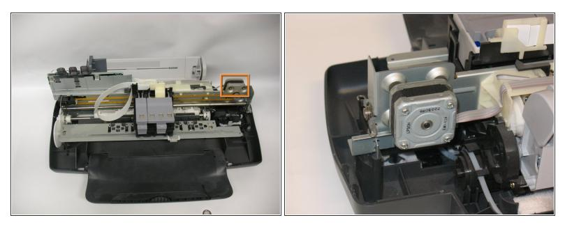
• Locate the drive motor. It is the square object located in the back right of the chassis.
