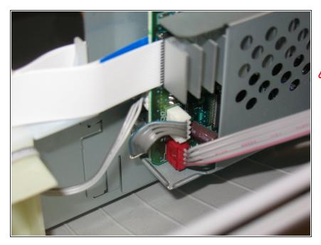
• Remove the red cable connecting the motor to the logic board.
