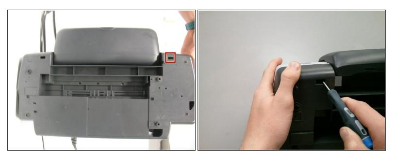
Insert the pointed end of a spudger into the hole on the bottom right corner of the printer and pry out the tab.
