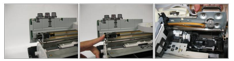
Push on the spring loaded tensioner on the left side of the belt to loosen the force on the drive motor.
