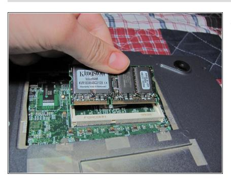
Remove the RAM from the socket and insert replacement RAM.
