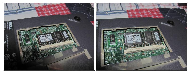
Carefully pull the tabs over the RAM chip down - the RAM will spring up.
