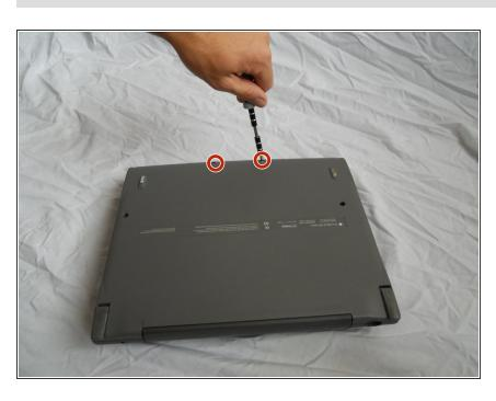
With monitor hinge at the bottom, remove the two top center screws.
