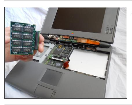
Once the old Memory board is removed, replace it with the new Memory board.
