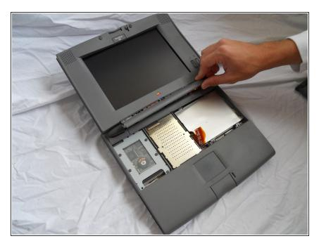
Remove the plastic panel on the bottom of the LCD Screen.
