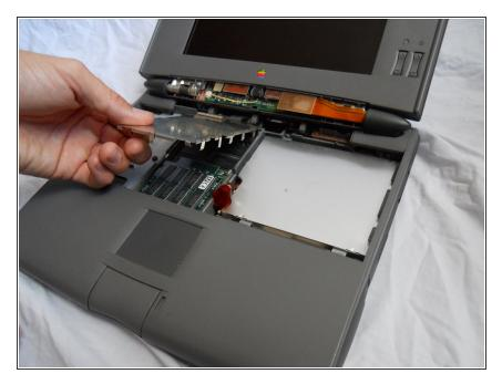
Remove the logic board protection plate.
