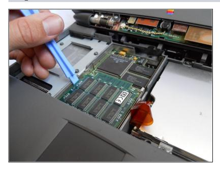
Using a plastic spudger, gently pry up the uppermost board fixture. This is the Memory (RAM).
