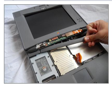
• Remove the plastic panel underneath the LCD Screen.
