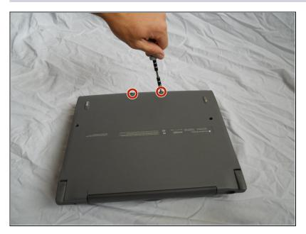
With monitor hinge at the bottom, remove the two top center screws.
