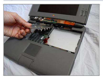
Remove the logic board protection plate.
