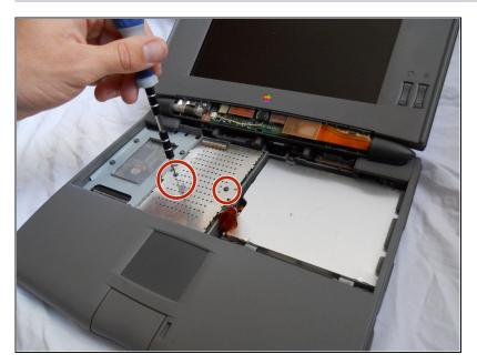
Remove the 2 T8 Torx Screws securing the logic board protection plate from the midsection of the logic board protection plate. Remove the T8 Torx Screw from the back of the plate, underneath the hinge.
