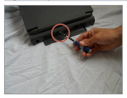
Open panel on back of the device. Remove 2 T8 torque screws.
