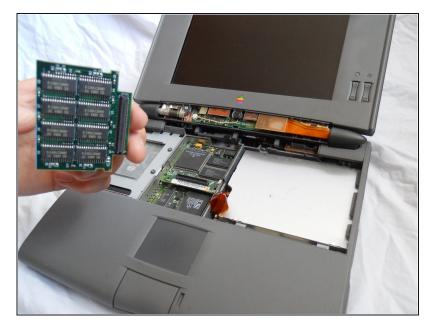
Once the old Memory board is removed, replace it with the new Memory board.
