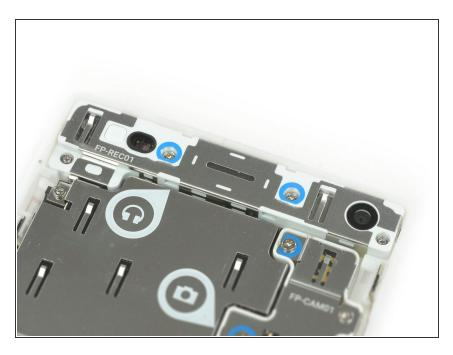
Remove the two Phillips #0 screws of the headphone module marked by the blue circles.
