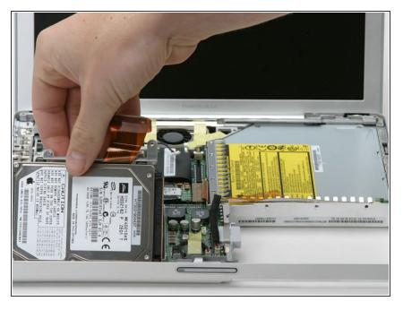
Use the orange cable to pull the hard drive up, then pull it and the hard drive bracket out of the computer.
