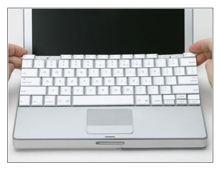
Lift the keyboard by the 'esc' and 'eject' keys and gently lift up until the keyboard is vertical.
