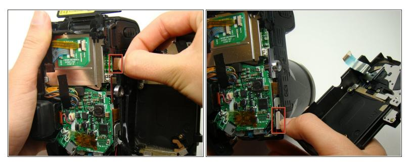
• Now gently unplug the two wires at the bottom of the panel.
