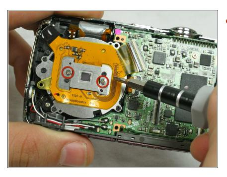
Remove the two 3.1 mm screws on the orange rectangular plate over the lens.
