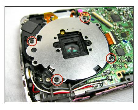
Remove four 3.4 mm black screws from around the perimeter of the silver plate.
