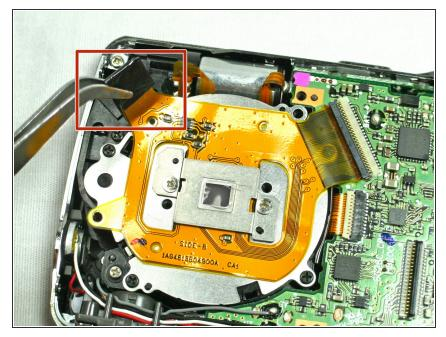
The black tape connecting it to the camera will lift up and allow you to release the left side of the rectangular plate.
