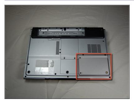
• With the battery removed, locate the hard drive access panel.
