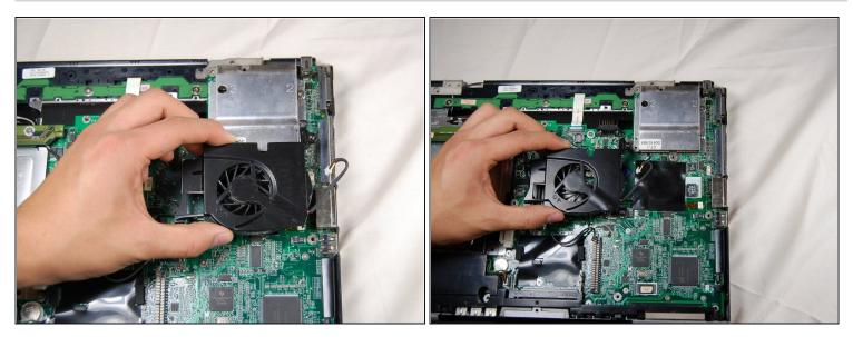
• With the wire removed, the fan should lift up easily from the board.
