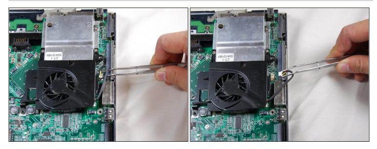
After removing the screw, use your <u>tweezers</u> to remove the wire connecting the fan to the board. Do not pull the fan out immediately or it may damage the fan and/or the computer.
