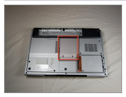
• Locate RAM access door on the bottom side of the laptop.
