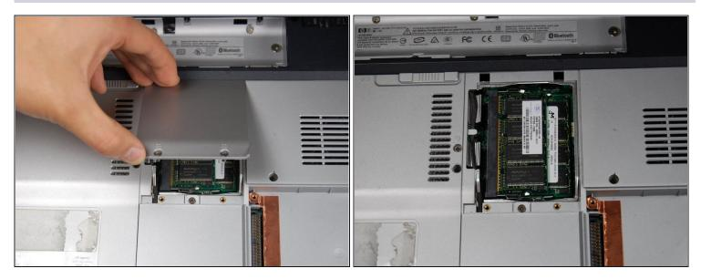
• Lift up on the screw side of the RAM access cover to remove it.
