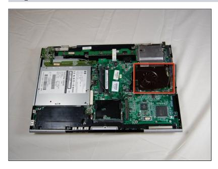
• With the back cover removed, locate the fan.
