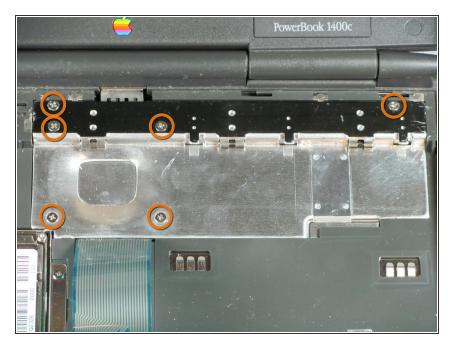
Locate the six screws that secure the heatsink.
