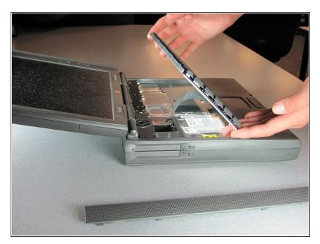
Gently lift the keyboard until only the ribbon cable remains attached.
