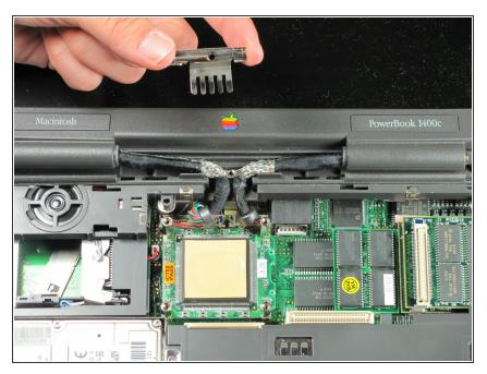
• Completely remove the metal cover.
