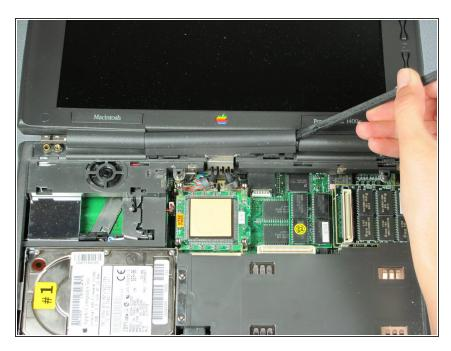
• Pry the center cap off by placing the spudger between the hinge and the center cap and prying upwards.
