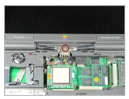
Identify the one 12.6mm long screw under the center cap.
