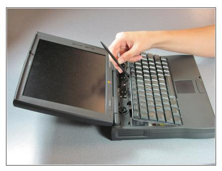
• Lift the keyboard up from the back using a spudger(wedge side).
