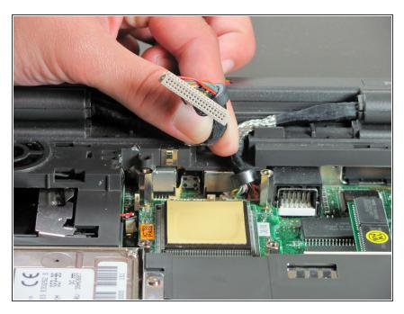
• Completely detach the left monitor cord from the logic board.
