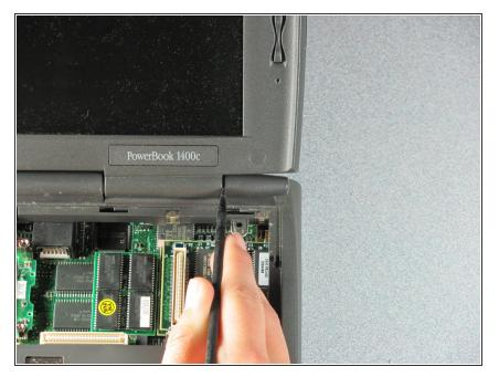
Pry off the end caps by putting a spudger between the monitor hinge and the end cap and prying outwards.
