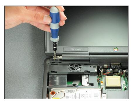
• Remove the 4 screws using the Phillips #0 screwdriver.
