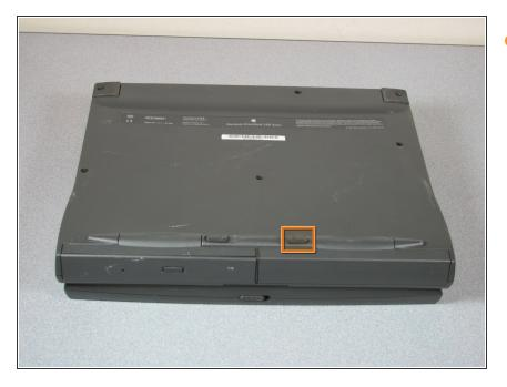
Turn the device upside down and then locate the battery latch near the front of the device.
