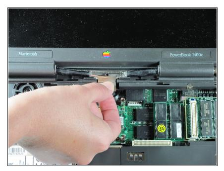
• Lift upwards on the metal cover under the screw.
