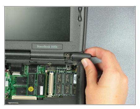
Once the end cap has been loosened by the spudger, pull outwards on the end caps.
