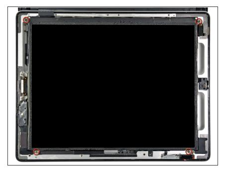
Remove the four 2.0 mm Phillips screws securing the LCD to the rear case.
